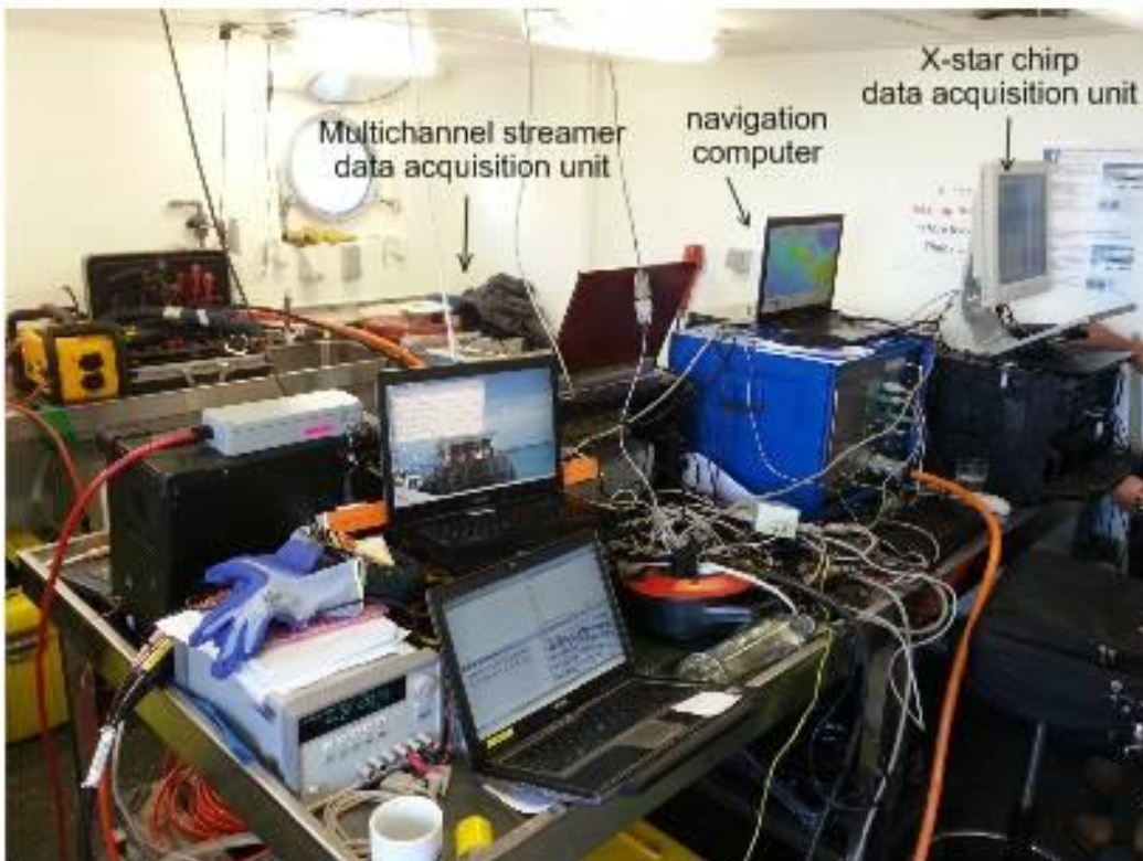
Figure 13 – Installation of the different acquisition and navigation recording units in the lab.
