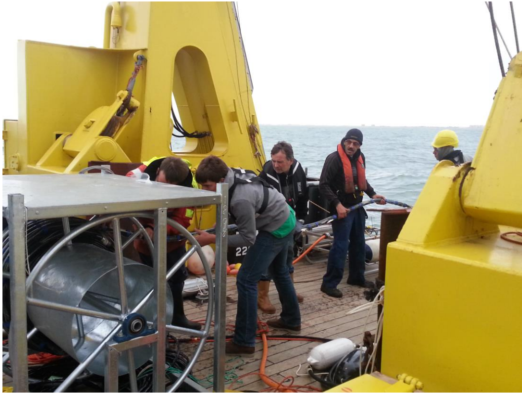
Figure 11 –Deploying the multichannel streamer from Deltares
